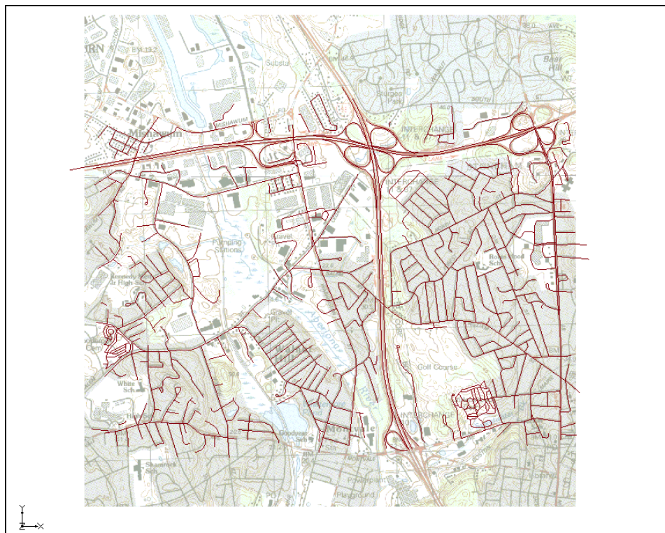
Figure 5 CAD data correctly positioned after specifying the projection
