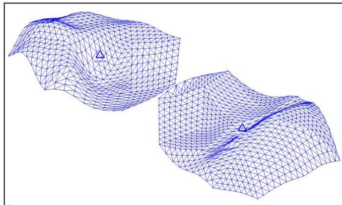
Figure 12 The sparse TIN and surface TIN
